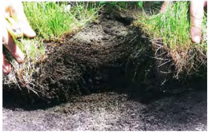
Deltalok root penetration exposed in a cut ecology bag
